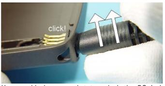
Use an old charger socket to unlock the DC Jack from the Grip Cover.
