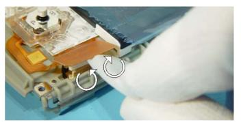
Remove Transceiver Keymat and unlock the Flexfoil Connector carefully.
