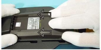
After the SRT-4 is taken away, the Grip Cover has to be unlocked from the A-Cover.
