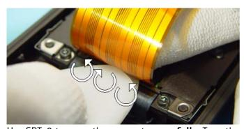
Use SRT-6 to open the connector **carefully**. Turn the opening tool several times to pull up the connector.
