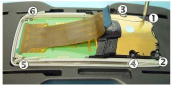
Unscrew six T6 screws in the following order. Assembly order is 3,4,5,6,1,2, with torque of 22Ncm.
