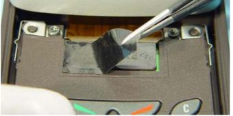
Remove the Protection Foil from the flex foil connector.
