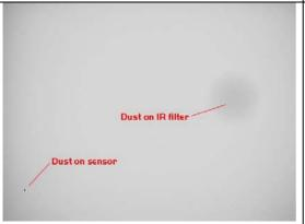
7. This distortion comes from camera dirt or dust, which can't be cleaned. Change Camera Module, if back window is clean.
