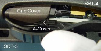
Press the levers so, that the nails of SRT-4 are between the covers and push it to the left forcefully.
