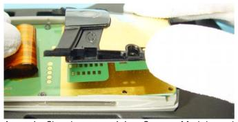
Acoustic Chamber, containing Camera Module and SIM Connector can be taken away now.
