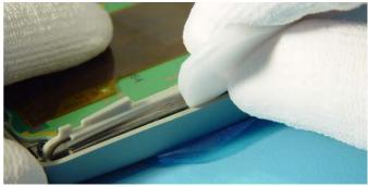
To separate Chassis from A-Cover, SRT-6 can be used to unlock the snaps on both sides along the edges.
