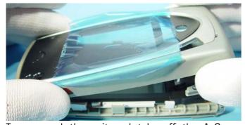
Turn around the unit and take off the A-Cover. Always protect windows and displays with protection foil to avoid dust and scratches.
