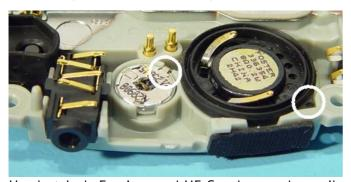
Headset Jack, Earpiece and HF-Speaker can be easily taken away. Note the guiding pins when assembling.
