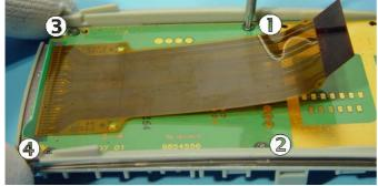
Radio Module LG4 is fixed with four T5 screws. Unscrew, using the shown order. Assembly order is the same (22 Ncm for all screws).
