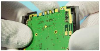
Gently press the edges of Keymat Cover and push off LS4 Module from the Keymat Cover.
