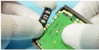
Take off the Battery Connector from LS4 Module.
