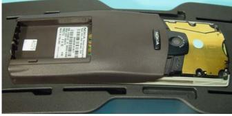
After removing Battery Cover and B-Cover use SRT 4 and SRT-5 opening tools for A-Cover and Grip Cover.
